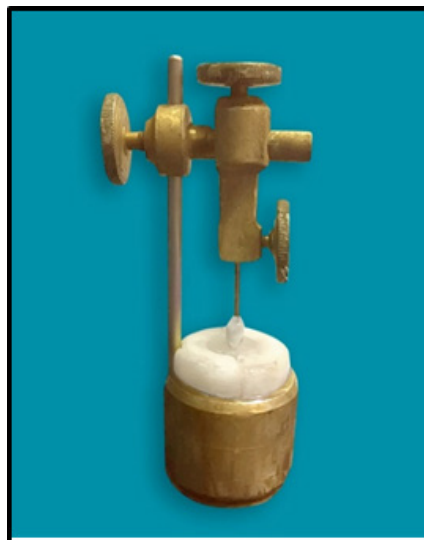
Figure 2: Showing abutment fixation in epoxy resin block using centralizing device.
